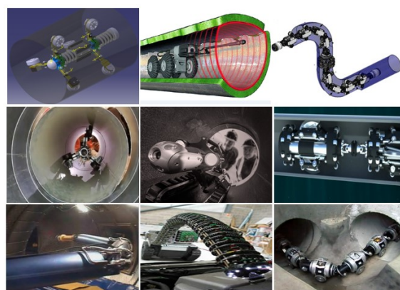
Figure 5 – Different constructions of service robots for inspection and control of piping systems [24,27,28]
